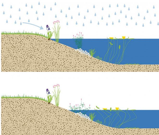
Section schemes with a higher water level (during rainfall) and with a lower water level. © atelier GROENBLAUW, Marlies van der Linden (based on: Geiger et al, 2009)
