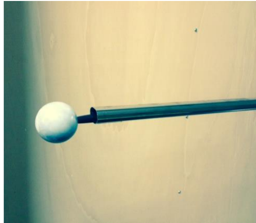
Figure 8 - The grey ball for the globe thermometer
