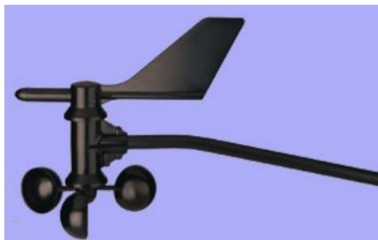
Figure 3 - Cup anemometer from the weather station
